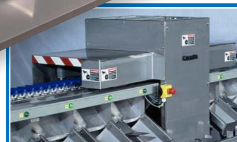
Optional: Additional cutting unit on the line to cut the asparagus to a preset length
