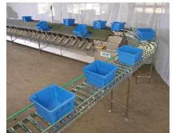
Transport belt on the line, roller conveyor curve, roller conveyor to remove full boxes
