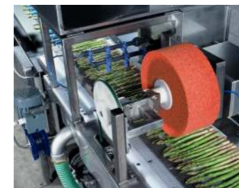
Small washing unit: The small version of the washing unit is sufficient if your asparagus is quite clean after having been harvested. This compact pre-cutting and washing unit has been designed especially to rinse any possible remaining dirt from green asparagus spears.
