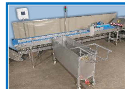
Floating basin in front of the infeed belt to facilitate the removal of the asparagus from the boxes as well as a waste removal belt system to collect and remove asparagus wastage from the cutting units
