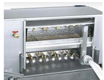
If the asparagus to be sorted is dirty, it needs to be washed from above and below by specially designed spray nozzles through the filter belt
