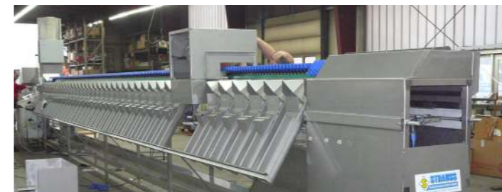
Open doors: Our grading software calculates the weight of the asparagus by its volume. The chutes are each equipped with a flap – „open door“ – that will open as soon as the predefined weight has been reached and transport the package into the collecting cup underneath.
