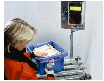
Scanner with display for the registration of harvest assistant, group of harvest assistants, harvest date and field which was harvested. The registration of these data enable the user to make an analysis per field and per harvest assistant
